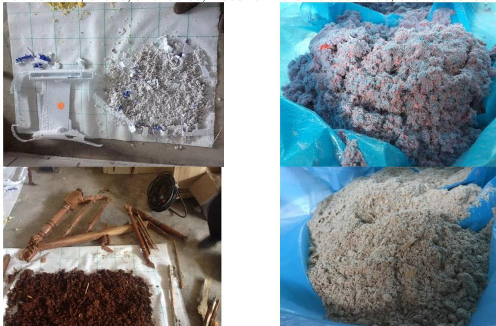
Figure 4. Plastic (up) and Wood(down) furniture before and after fragmentation
