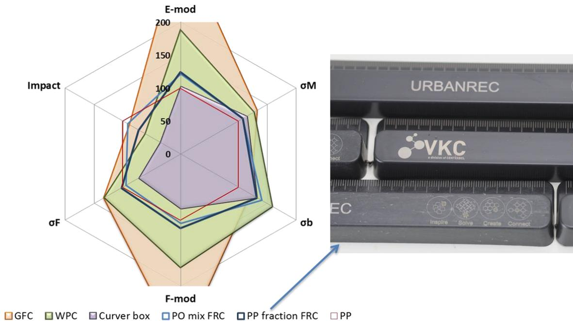
**Figure 5 Radar plot comparing the mechanical properties\* of the recycled plastics FRC's to unfilled, virgin PP and to virgin WPC and GFC (left) and illustration of the demonstrators produced from the PO mix FRC (right).**
